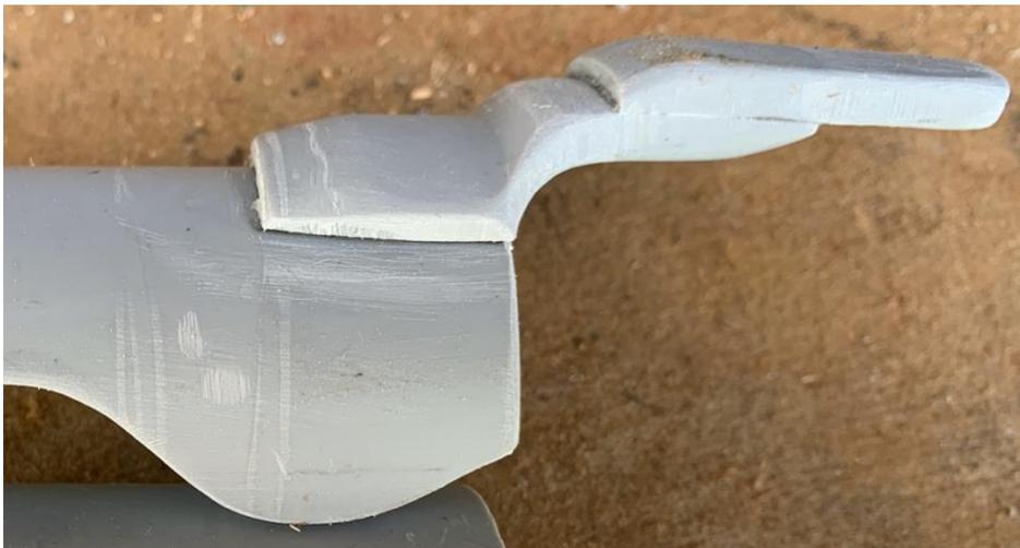
You must glue a piece of scrap conduit to the top of the arm to give it the right height and length to reach the thumb throttle.
