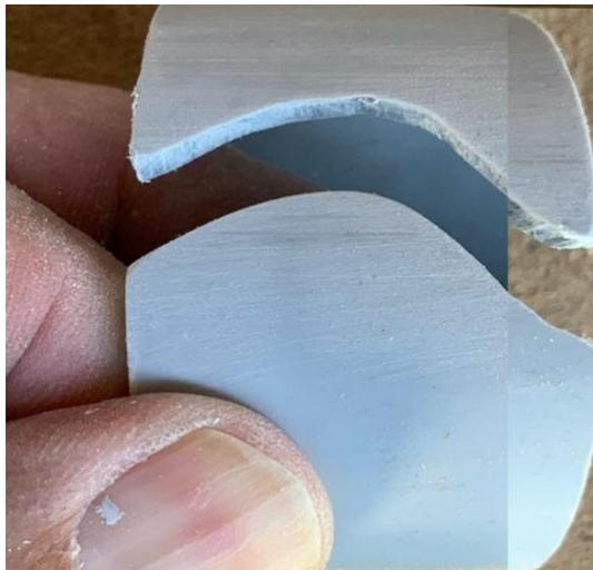
Cut the piece of conduit down each side. I chose to create a wavy line to provide greater strength when the two halves are rejoined over the bike's handlebar grip.
