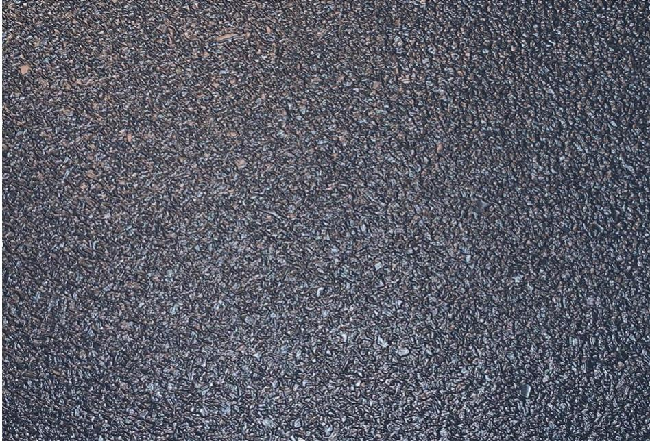
Here's the material I used to wrap around the axillary grip throttle. One side has non-slip material, the opposite side has an adhesive backing. When applied, it holds the two halves of the axillary grip together, while simultaneously providing an excellent grip surface.
