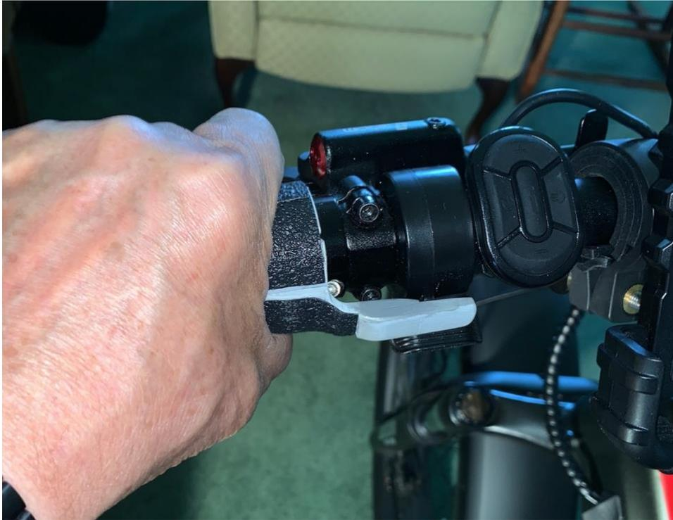
An arm on the axillary grip throttle engages the bike's thumb throttle. The spring in the thumb throttle will help rotate the axillary throttle.
