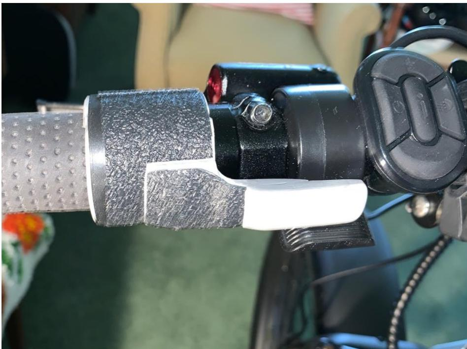
Here's how the axillary grip throttle looks when installed. When using the device, the arm of the axillary twist throttle rests on top of the thumb throttle.
