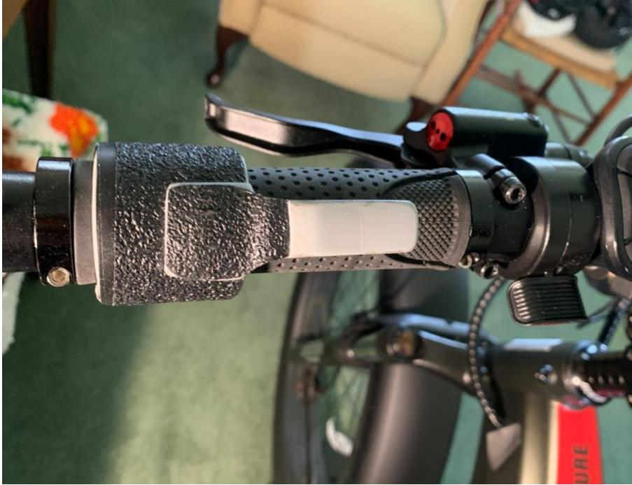
When not in use, you should slide the axillary grip throttle to the left. This will separate the arm from the thumb throttle.
